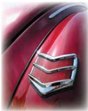
The distinctive chevron taillight. The '40 Standard came with just one on the left side. It functioned only as a brake and running light, not as a turn signal.
